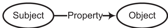
Figure 3 Graph model for an RDF statement. An RDF statement can be modeled as a DLG with resources (subject and object) as nodes and properties as the edge connecting from ‘subject’ to ‘object’.
